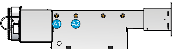
Figure 22. Water connection on the right-hand side (R).
