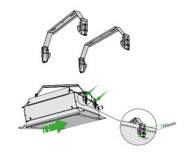
Figure 19. Installation with quick bracket PARASOL Z QUICK SUSPENSION KIT
