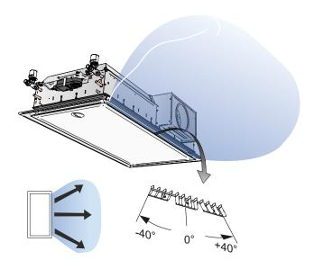
Figure 8. Possible settings for the ADC, Fan-shape
