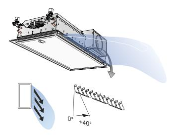
Figure 9. Possible settings for the ADC, X-shape
