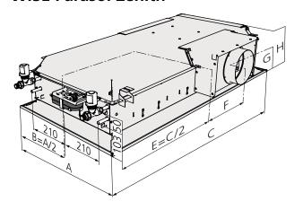
Figure 24. Dimensional drawing - long side connection (the length 1200 with air connection on side 2 is shown in the example).
