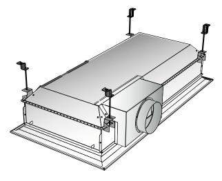
Figure 17. Suspension double-module units
