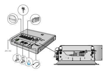
Figure 1. Components that are factory fitted on WISE Parasol Zenith A: Commissioning button
