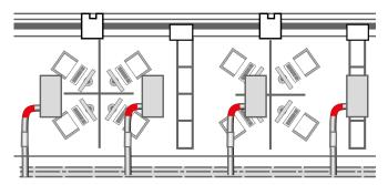
Figure 14. Installation example. Straight air connection, alternative with 90° bend.
