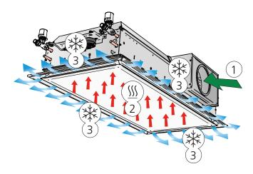
Figure 4. Variant A: Cooling and supply air function
