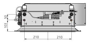
Figure 21. Dimensions, water connection length 600, 1200, 1800
