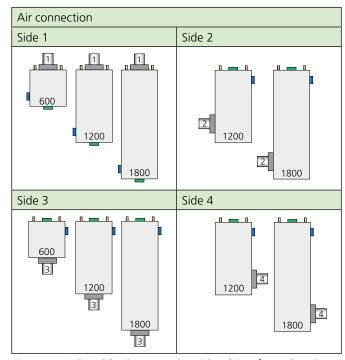
Figure 16. Selectable air connection sides, (view from above).
