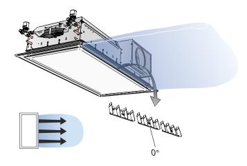
Figure 10. Setting options ADC, Straight setting
