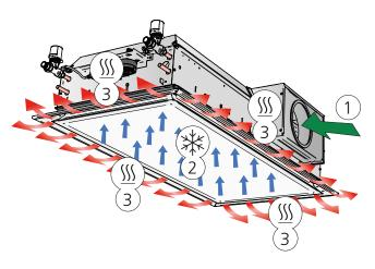
Figure 5. Variant B: Heating and supply air function (also including cooling function)
