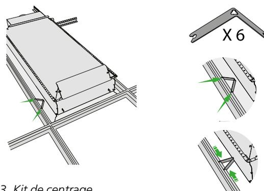
Figure 23. Kit de centrage SYST CENTERING KIT PARASOL
